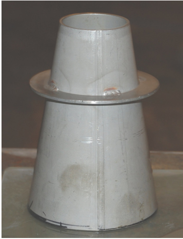
Figure 2 Left figure shows the mini slump cone and right figure shows the final spread of a micro mortar in the mini slump test
