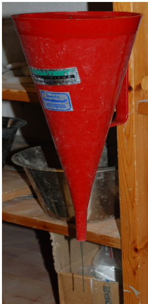
Figure 3 A Marsh cone. The time needed for the sample to flow out of the cone is measured.
